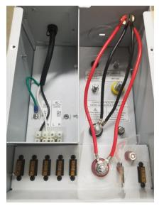
**Step 6:** Connect the two sets of positive and negative wire ends from the 6-inch cables to the "Solar Input" terminals of the two ZENITH controllers as shown below.
