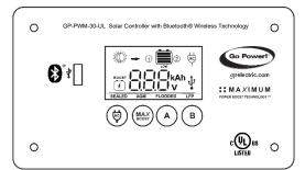
If the GP-PWM-30-UL experiences a battery over voltage (>15.5 VDC) on battery bank 1, the controller will stop operating, and the display will begin to flash with all icons. The controller will resume operating when the voltage drops to a normal level <15.5 VDC.
