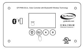
To activate, hold the MAX BOOST Button for 3 seconds. As long as there is full sunlight present, your battery voltage will be boosted (to 14.4 VDC for Flooded, AGM and LFP; and 14.1 VDC for SEALED/GEL) for 30 minutes regardless of the battery's state of charge.
