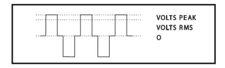
FIGURE 1: D/A INVERTER-MODIFIED SINEWAVE
