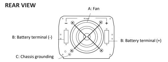
A: Fan: Do not obstruct, allow at least I inch for air flow.
