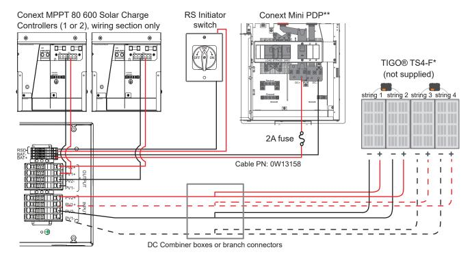
\*IMPORTANT: The Rapid Shutdown functionality is achieved only when the PV modules are equipped with compatible models of TIGO® TS4-F, installed according to local codes and standards.
